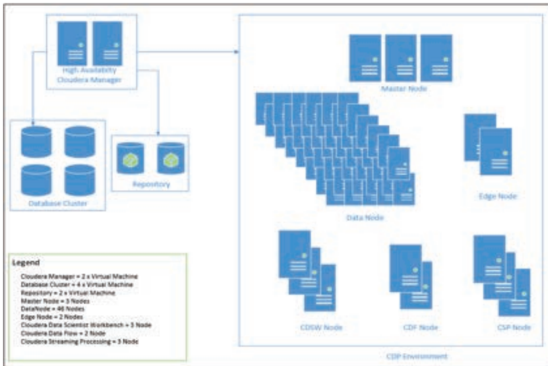
Figure 3.13: IWSDC Data Lake Ecosystem Design Diagram (1/2)
